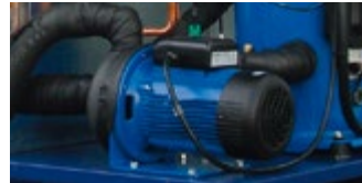
Standard Pump P3 (3 barg); optional P5 pump (5 barg).
