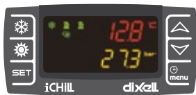
IC208CX sophisticated microprocessor connectable to supervisor systems through RS485.
